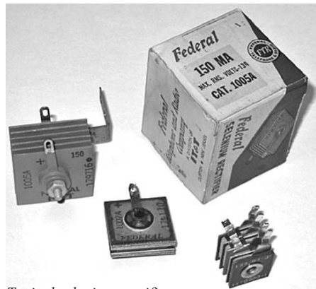
Typical selenium rectifiers.
