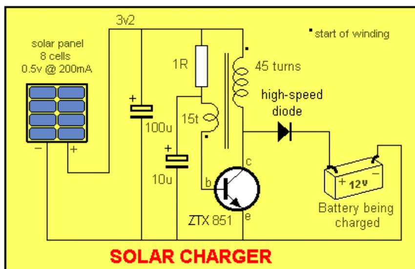
The aim of this project is to cater for the other end of the range. We are looking at charging a 12v battery, using the cheapest set of solar cells and the cheapest inverter. This also means the cheapest 12v battery - a 1amp/hr gell cell or 6v cells salvaged from old analogue mobiles!
