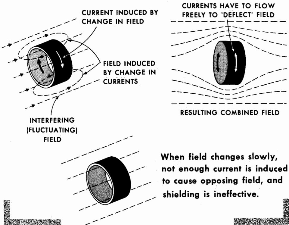
Outside the shield, the two fields are in the same direction and the combined magnetic field is increased. Therefore, this kind of shield has the effect of "pushing" the inducing field outward, instead of permitting it to reach the shielded circuits. Because it depends on fluctuating fields, this kind of shield is completely ineffective against steady magnetism. It is also comparatively ineffective against low-frequency fluctuation, and only becomes really effective at higher frequencies.
