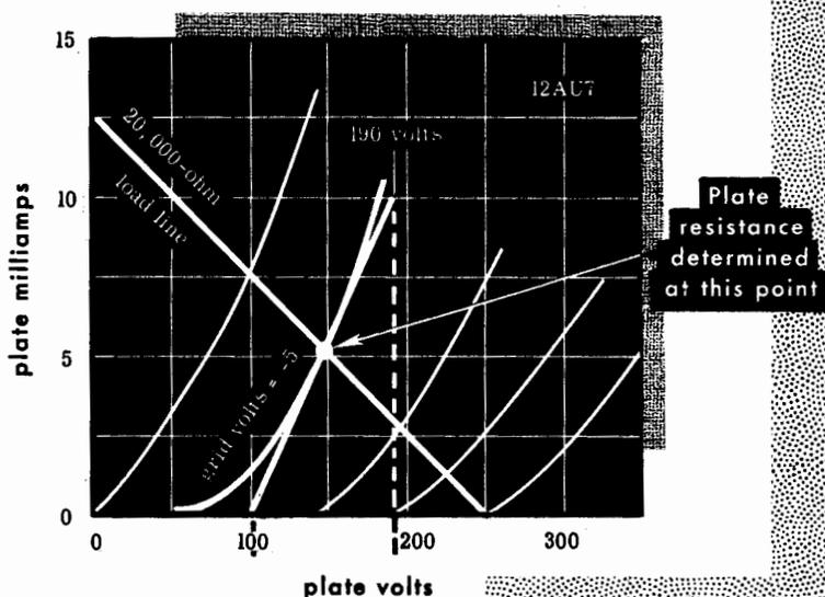
By laying a straight-edge (ruler) along the curve at the point where the two lines cross, its slope at *this particular point* can be found. Extending the line drawn as tangent to the curve down to the zero current line and up to the 10-milliamper line, the corresponding voltages may be read off and the plate resistance calculated.
