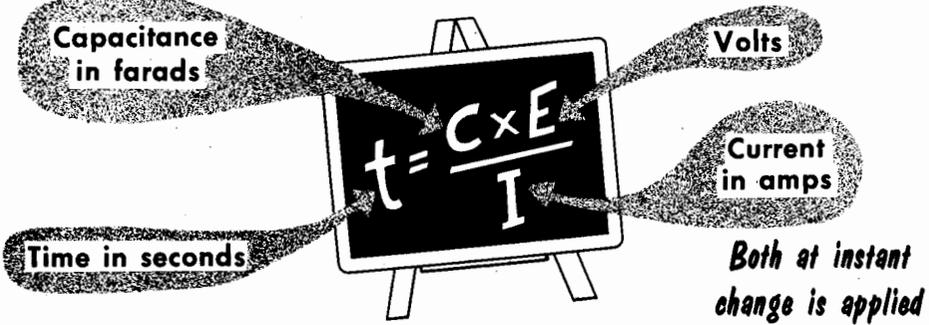
A Time Constant is the time required for a capacitor to charge to 63.7% of the applied voltage
