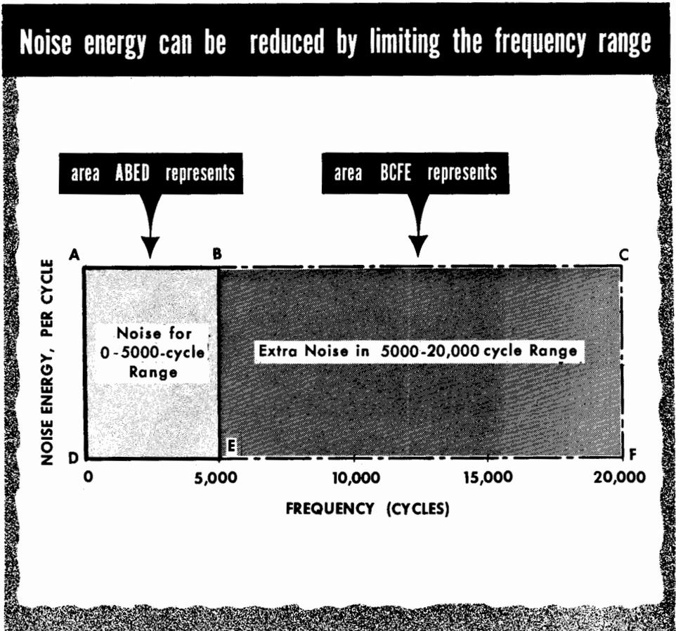
At an average room temperature, the noise energy of any resistor is .0165 micromicrowatt, or .000 000 000 000 000 0165 watt, per cycle. If we take the bandwidth as 10,000 cycles, the noise energy will be 165 micromicrowatts. Once we know the value of the resistance, we can calculate the noise *voltage* it will produce, by the usual formula,  $E = \sqrt{P \times R}$ . For example, for a 1-megohm resistor (1,000,000 ohms), the noise voltage for a bandwidth of 10,000 cycles is:
