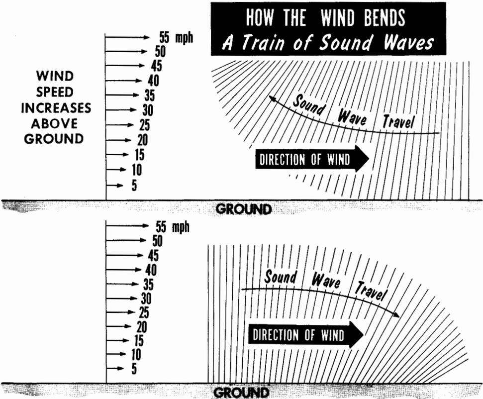
The wind travels at different speeds at various heights above ground. Air in contact with the ground hardly moves at all, but the higher you go, the stronger the wind. For this reason, the higher part of the sound wave traveling *with* the wind moves faster than the part near the ground. (The wind speed is added to the normal speed of sound.) This makes the wave lean forward, and bear down on the ground, and the sound heard here is more intense than without the wind.
