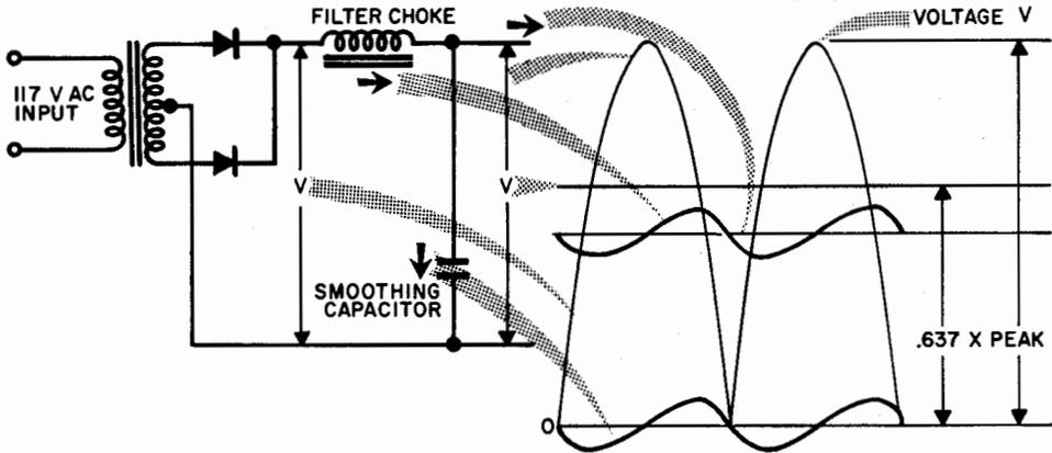
**THE OUTPUT OF A CHOKE FILTER
