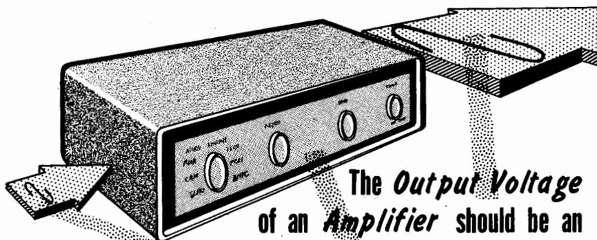
The Output Voltage of an Amplifier should be an exact replica of the Input Voltage only Much Larger.
