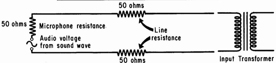
1. If input transformer primary is for 150 ohms, step-up will be 5 db less than for 50 ohms.
