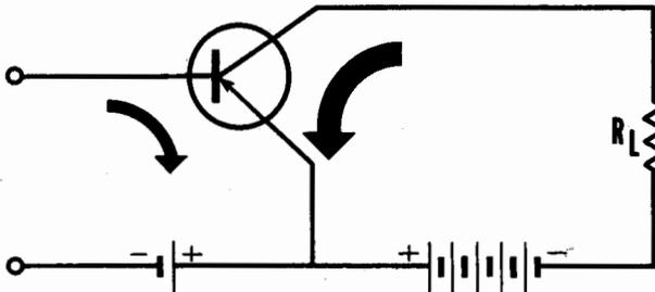
A small voltage and current change in the base circuit produces a much larger Voltage and Current Change in the collector circuit.
