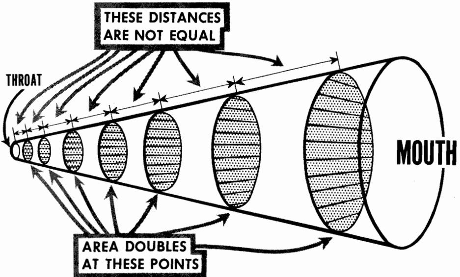
**Area inside a cone-shaped horn does not double at constant changes in distance along the cone. Therefore the sound waves do not expand at a constant rate.**
