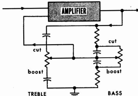
By combining the arrangement and using a potentiometer across the two capacitors, we provide a continuous adjustment that will go from bass boost to bass cut. Most modern tone control circuits combine the two arrangements with two controls, one for the treble boost and cut, the other for bass boost and cut.
