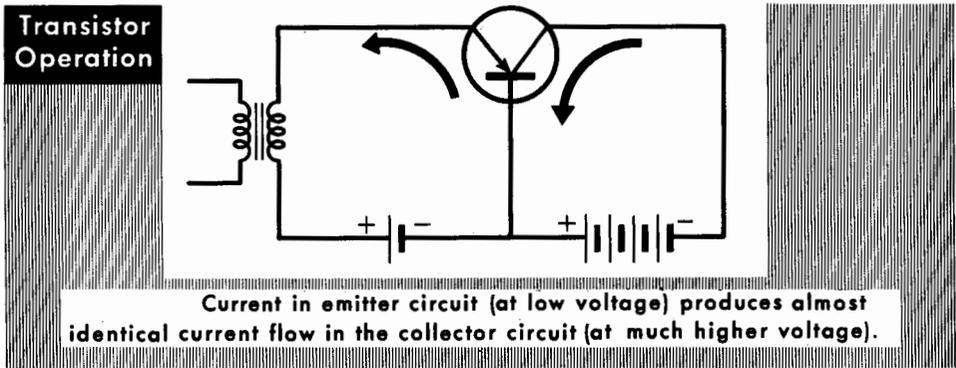
However it is made, the transistor works by having a potential applied to the electrode called the *collector* in the direction *against* the normal flow of current for this kind of device. (Either of the junctions between the electrodes and the base would act as a rectifier allowing current to flow one way but not the other).
