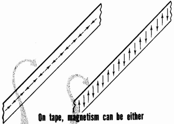
On tape, magnetism can be either lengthwise or crosswise. Lengthwise is most used.
