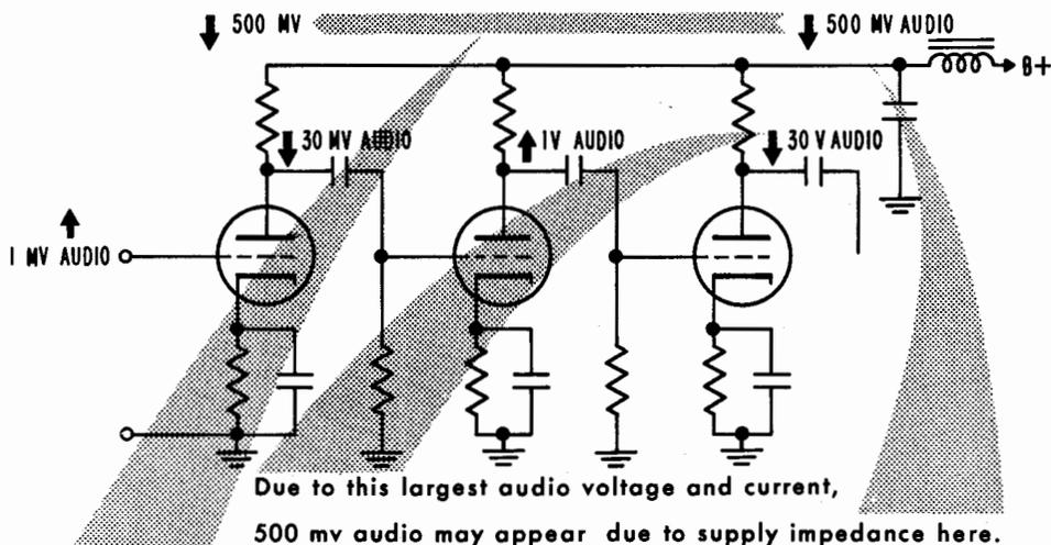
This voltage gets fed back and is in right 'phase' to add to original 30 mv at this plate, probably causing oscillation. This also may be avoided through the use of decoupling resistors and capacitors.
