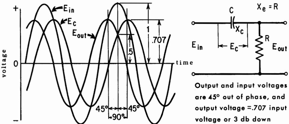
Notice that making the two voltages ( $E_c$  and  $E_{out}$ ) equal does not mean that either of them is equal to *half* the input voltage ( $E_{in}$ ), because there is a  $90^\circ$  phase angle between the voltage across the capacitance and that across the resistance. For this reason, the two voltage drops cannot be added arithmetically.
