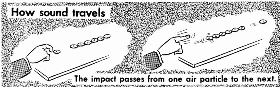
The natural speed, or propagation velocity, of sound is controlled by two properties of the air through which it travels:
