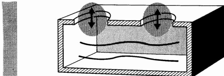
In a box with two holes, the air in the holes moves together
