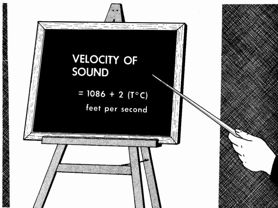
At 20° C (normal room temperature), sound travels at  $1086 + (2 \times 20) = 1126$  feet per second.
