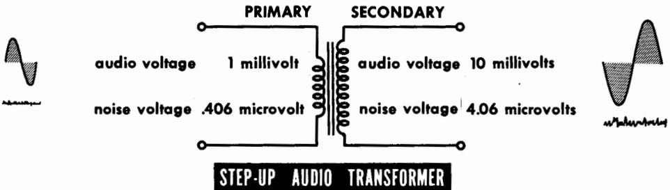
When a transformer is used to step up the audio voltages from a microphone or pickup, it steps up the noise voltage that comes with it. Suppose the audio voltage is 1 millivolt, and the resistance of the microphone or pickup is 500 ohms. In a bandwidth of 20,000 cycles (which we expect for high fidelity), the noise voltage from 500 ohms is
