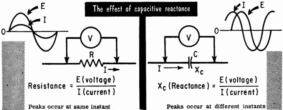
When the reactance of a capacitor is equal to the circuit resistance, the voltage across it is equal to that across the circuit resistance. At this frequency the phase between the input and output will be  $45^\circ$ , and the voltage output will be 0.707 of the voltage input or 3 db down.
