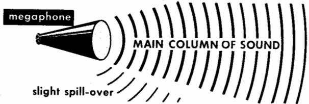
The directivity of a horn is dependent on its precise shaping. For example, a shape called the *tractrix*, which is nearly identical with the exponential shape, except at the mouth, is designed to produce hemispherical waves; in other words, to cover the entire 180° in front of its mouth. This ideal distribution from the tractrix only exists at the lower frequencies it radiates. At higher frequencies, the bell has progressively less effect.
