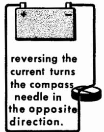
If you suspend a magnet or a compass needle over a wire connected to a battery, the needle will swing to one side. If you reverse the current in the wire, the magnet (or needle) will swing in the opposite direction.
