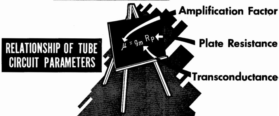
If there is no coupling resistor present (this was the case when we first examined the circuit), the voltage remains constant, and the current fluctuates. The plate current fluctuation for each volt of grid fluctuation is the transconductance of the tube. The relationship between these two conditions (which have no practical use, but help no end in figuring out the operation of practical tube circuits) is determined only by the parameter that we have called plate resistance.
