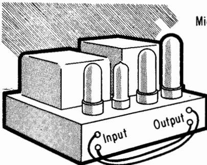
IF AN AMPLIFIED OUTPUT FEEDS BACK TO THE INPUT, IT WILL OSCILLATE.
