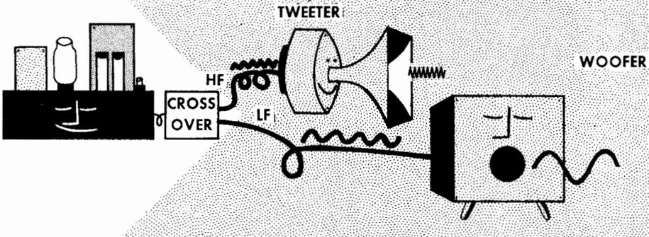
If the low frequencies are fed to a unit not designed to accept them, it will rattle and distort badly. Feeding frequencies higher than a unit is intended to handle will not cause any particular distortion, but will result in loss of power at these frequencies, because the voice coil will accept the power, although incapable of delivering corresponding sound waves. For this reason, *dividing networks* are needed so each unit gets “what is coming to it.”
