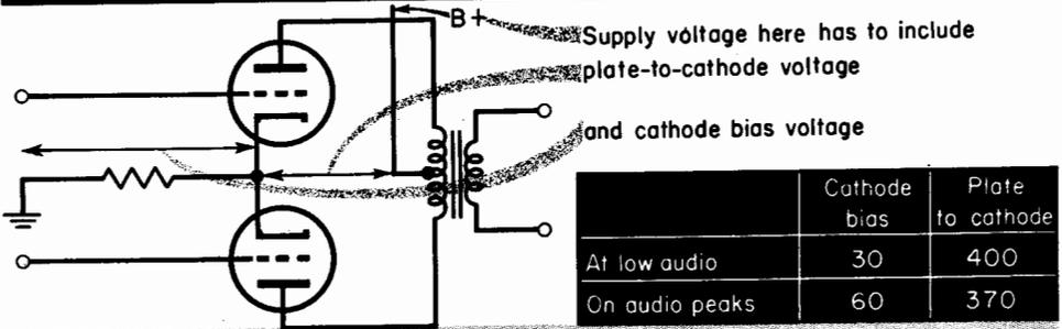
**NOTE:** This table assumes that B+ does not drop with increased current demand. If it does, reduction in plate-to-cathode voltage on peaks is even worse.
