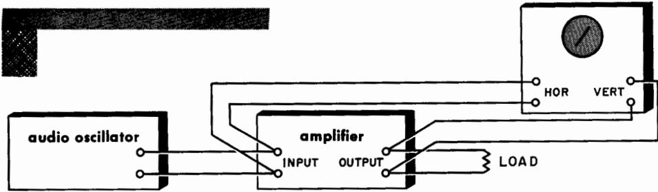
SCOPE TRACE IS A STRAIGHT SLOPING LINE IF OUTPUT IS ALWAYS A PROPORTIONATELY AMPLIFIED VERSION OF THE INPUT
