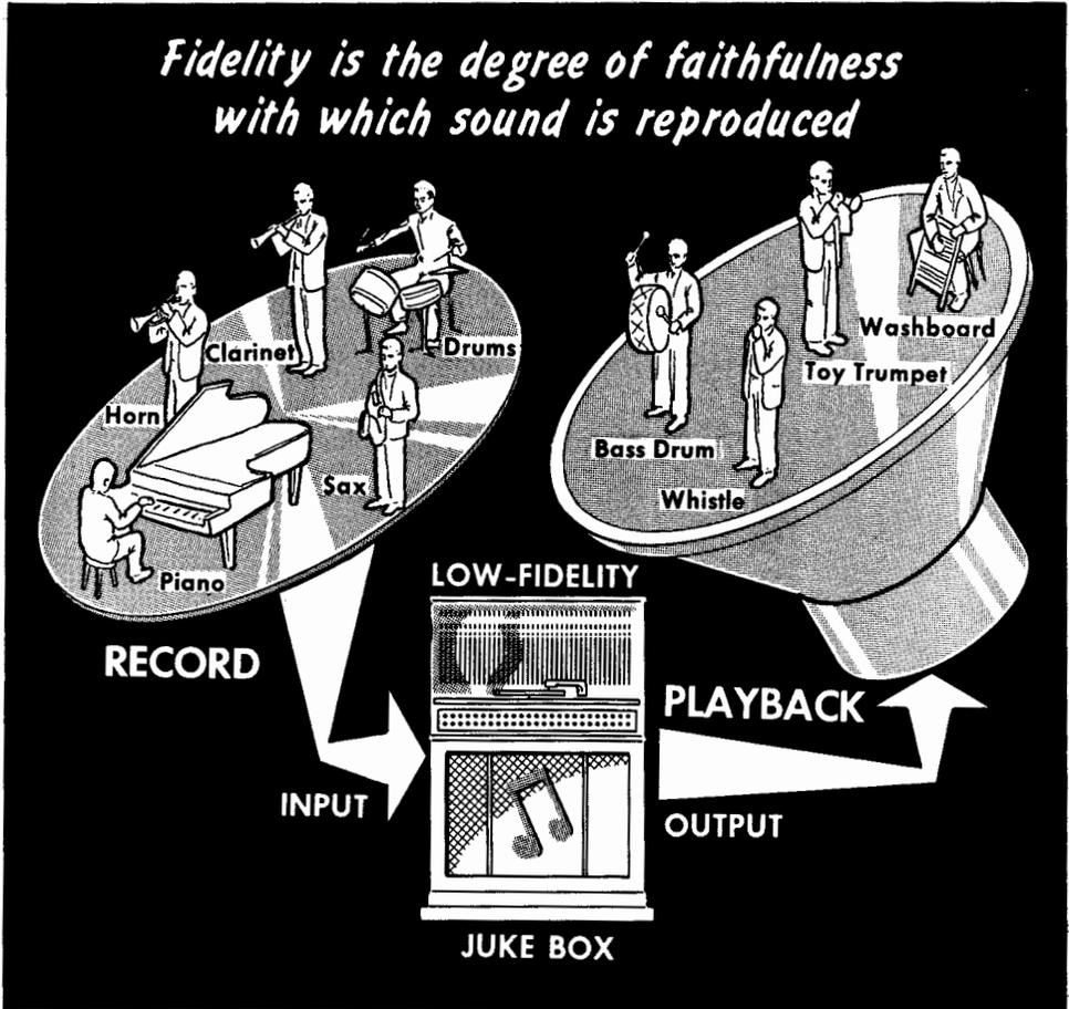
The faithfulness with which the sound reproduced through a loudspeaker copies the original is called the *fidelity* of the system. If all the original frequencies are present in their original proportions, the system has "high fidelity." In the average juke box—especially the older ones—the fidelity is very low. The tune, of course, can be recognized, but you would have difficulty in recognizing some of the instruments playing it.
