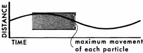
THIS shows how each air particle moves back and forth... These very small movements passed
