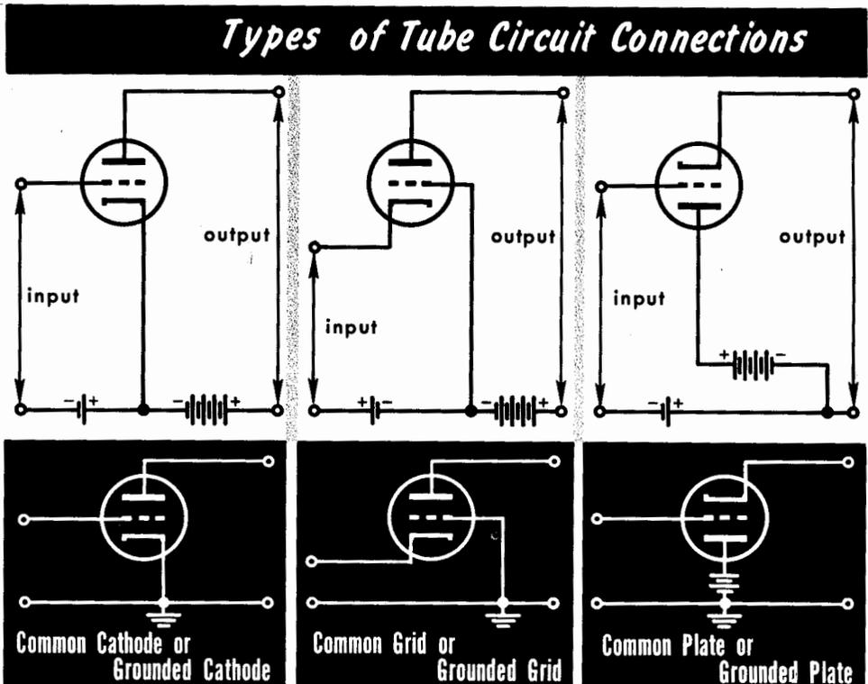
We encounter one more expression for this: because the point to which measurements are all made is *common* to both input and output circuits, this is called a common point. The way of working a tube we have described is called *common cathode*, or *grounded cathode*.
