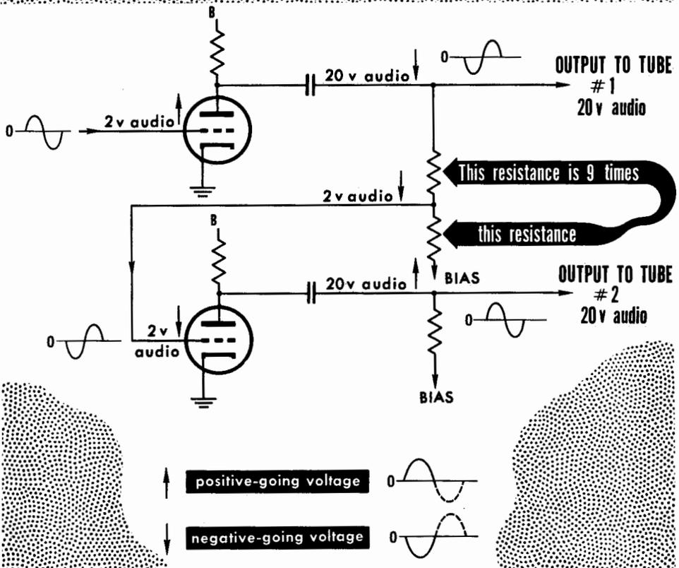
A positive fluctuation of 2 volts at the grid of the first paraphase tube produces a negative fluctuation at its plate of, say, 20 volts, which appears at the grid of one of the output tubes. This 20-volt fluctuation is also divided to provide a negative fluctuation of 2 volts for the grid of the second paraphase tube and becomes a positive fluctuation of 20 volts at the plate, providing positive fluctuation for the grid of the second output tube.
