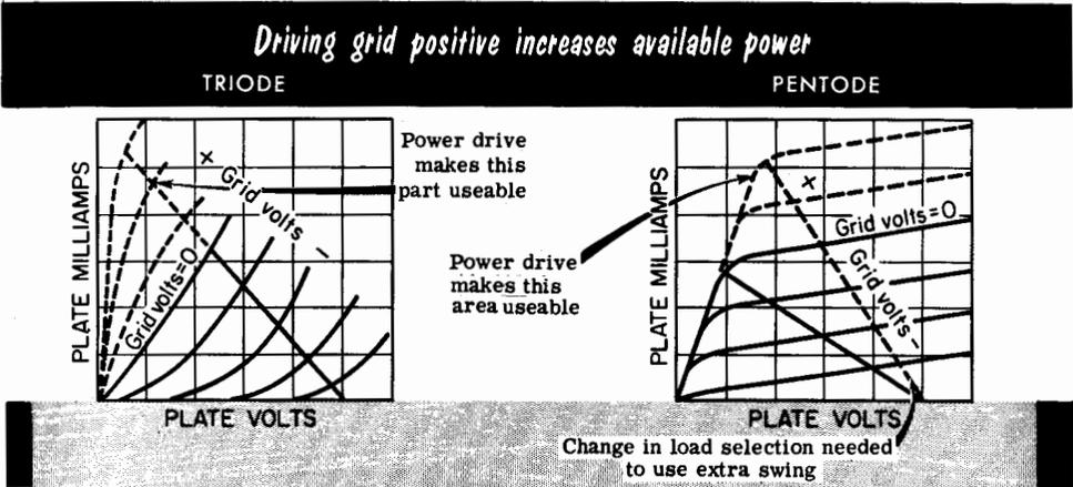
One more thing can be done to increase the power available from a given pair of tubes. If the control grid is made positive, the plate current will rise still farther, whether a tube is operated as a triode or pentode. In the case of pentode operation, the load value must be changed, otherwise additional grid swing into the positive cannot extend the *length* of the load line. This would still result in clipping that no amount of grid current could remedy.
