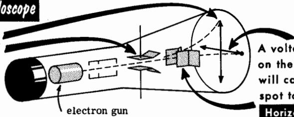
A voltage applied on these plates will cause the spot to move
