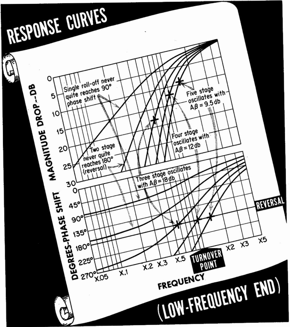
In this way the gain is reduced at the rate of 6 db for every octave with only a little more than 90° phase shift (because the other rolloffs are gradually starting) so it gets the magnitude of  $A\beta$  down to much less than 1 before the phase shift reaches 180°.
