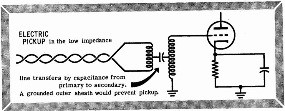
Although electric pickup is not important to the low-impedance circuit itself, it *can* be transferred from the primary to the secondary of the transformer by the capacitance between windings. Use of an outside sheath as an electric shield will help prevent this.
