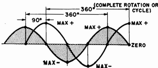
VOLTAGES  $V_2$  and  $V_3$  are always displaced in time by a "phase" of  $90^\circ$
