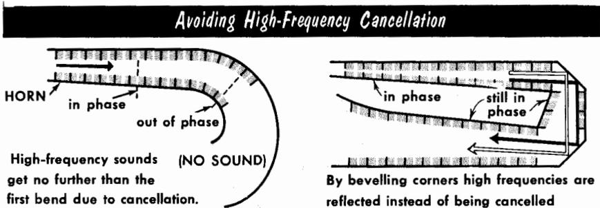
One way in which to compensate for this problem is to design the bends of the horn so as to “invert” the waves at higher frequencies, thereby equalizing the path lengths. Instead of following a smooth contour at the corners, the shape is arranged to reflect the complete wave.
