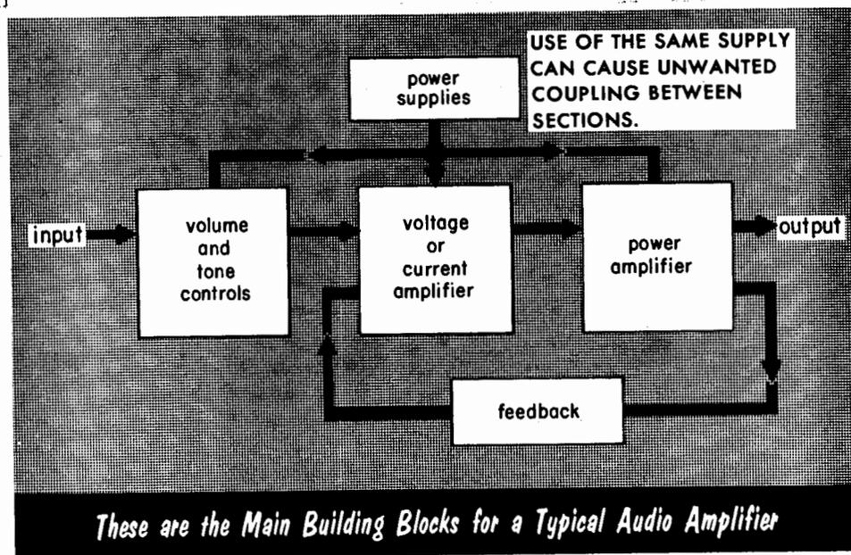
Finally, you need certain controls, volume, and tone, as well as equalization. These have to be put outside the main feedback loop, although they may use some feedback of their own. But if you make the mistake of putting feedback around a volume or tone control, the feedback will carefully undo all the effect of the control! It holds the gain steady, and has no means of knowing that you *meant* it to change.
