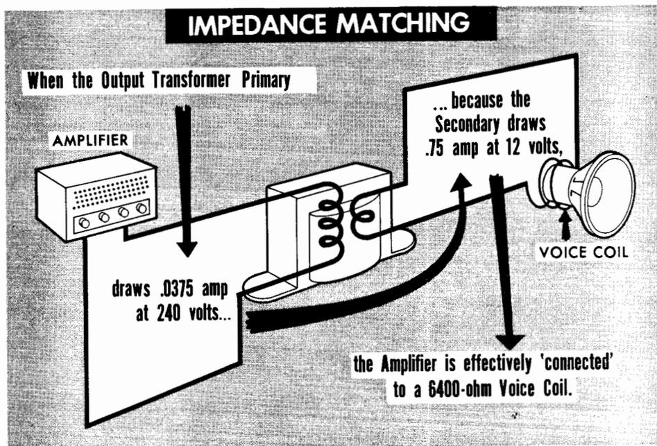
When the amplifier supplies 240 volts to the "high" winding of the transformer, the core will be magnetized, and, due to its high inductance, very little current will be drawn from the amplifier, unless the voice coil is connected to the low winding.
