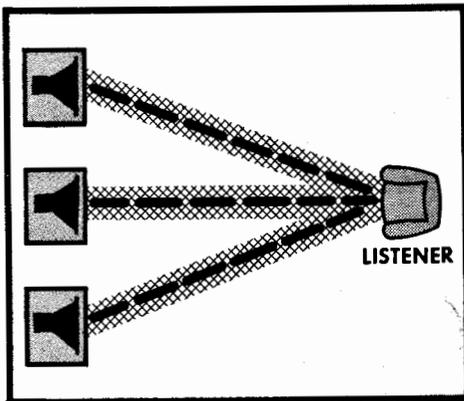
Using a 'dead' room eliminates playback room reverberation but the recorded reverberation comes with the original sound, which is still not natural.
