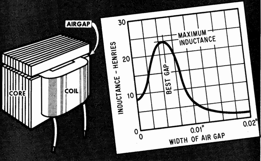
Using too small an air gap, or no air gap at all, means the primary current will cause the core to saturate and thus the inductance will practically disappear. Using too large an air gap amounts to making the transformer almost air cored, which again will result in a very low inductance. There is always an optimum size for the air gap, which will result in the biggest practical value of inductance for a transformer that carries direct current in one of its windings.
