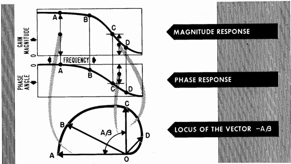
The loop gain  $A\beta$  is the important thing to consider. We can draw a series of lines from a starting point called O (for Origin). Each line represents both the magnitude and the phase angle of  $A\beta$  for a different frequency. Joining the outer ends of these lines produces a curve that represents all possible positions for the tip of the  $A\beta$  vector and shows how  $A\beta$  varies in phase and magnitude due to frequency changes. This curve is called a Nyquist diagram.
