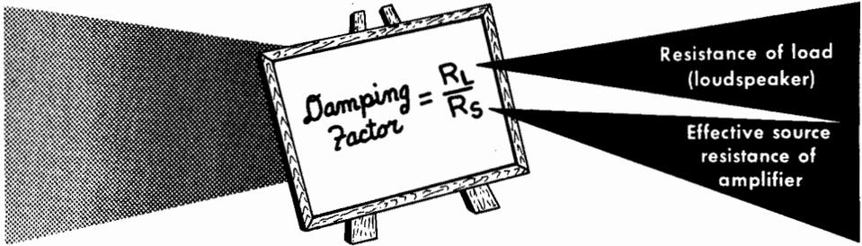
The use of a high damping factor (or a low source resistance) cannot do everything. The electrical damping has to act on the motional impedance of the loudspeaker. (Motional impedance is the impedance reflected back to the loudspeaker terminals due to the movement of the diaphragm.) This impedance is only a small fraction of the total impedance of the loudspeaker, most of which is due to the resistance and inductance of the voice coil.
