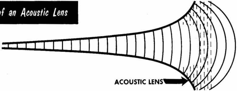
The best solution for wide ranges of frequency is the acoustic lens (a series of perforated or parallel plates). Like its counterpart in waveguide radio, it is effective *above* a certain limit frequency. As the ordinary horn construction, using a tractrix or similar mouth, can be effective *up to* a frequency where the bell ceases to have effect, the lens can be arranged to take over from there and effectively scatter all frequencies above that point.
