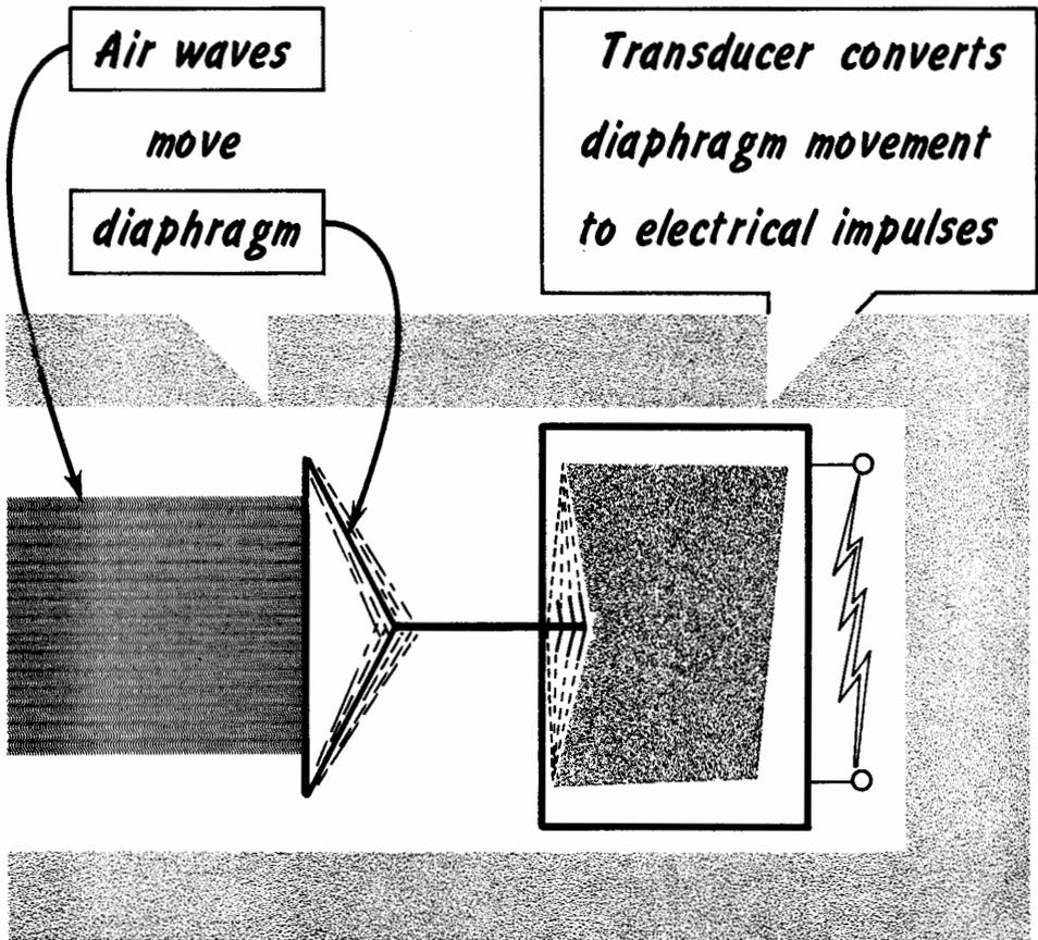
Every microphone has two basic actions: first to convert the acoustic vibrations of the air into mechanical vibrations by having the air move a diaphragm—a light stiff surface; second, it must act as a *transducer*, and convert this movement of the diaphragm into electrical currents or voltages. One important difference between microphones is the arrangement used for making this conversion.
