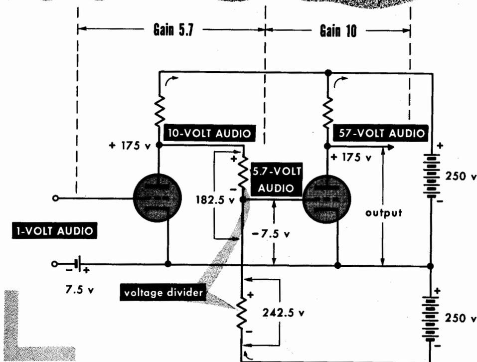
Another system that uses resistance coupling has just two supplies, one positive and one negative. To bring the voltage at one plate down to a suitable level for the following grid, two resistors are used as a voltage divider. Of course these resistors will divide the available fluctuation at the plate as well as dropping the steady voltage.
