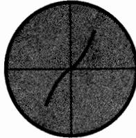
Two curved traces indicating wrong amplifier loading. Both are distorted sine waves.
