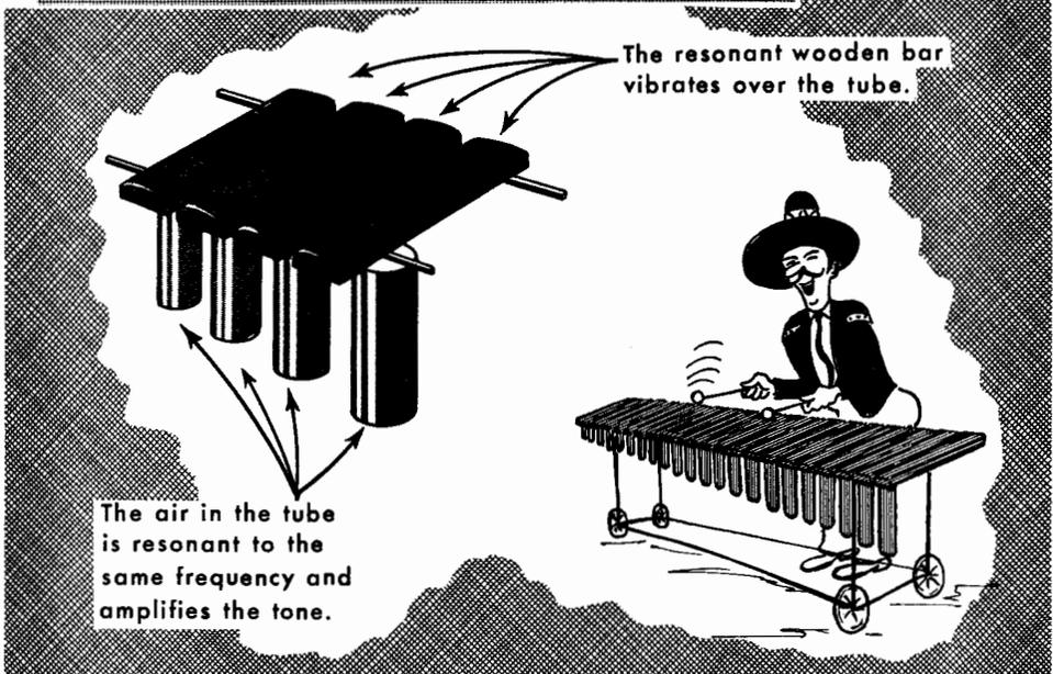
With all these musical instruments, it is a family of resonance patterns that control the production of tones peculiar to that instrument. In the xylophone or marimba, a vibrating piece of wood initiates the tone, which is reinforced and given its fullness of tone by a resonant tube, in which an air column is set in vibration by the feeble vibrations from the wood bar.
