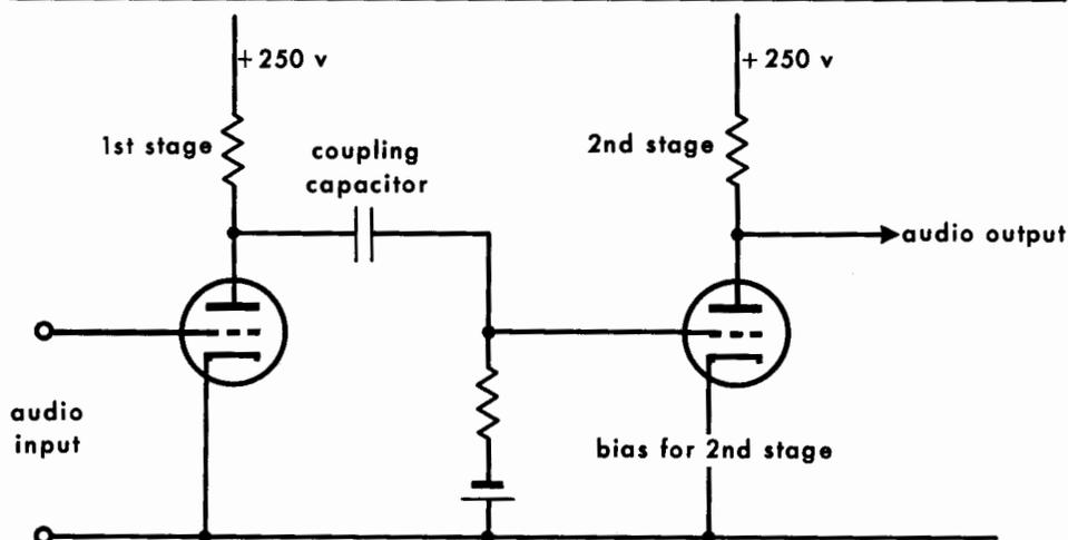
**The COUPLING CAPACITOR prevents the d-c voltage from reaching the grid of the next stage while passing on the audio fluctuations**
