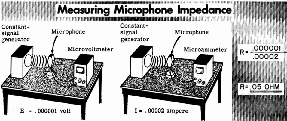
Thus the real impedance of .05 ohm has been multiplied by 12,500 .05, or 250,000. The impedance matching ratio 250,000:1 is the square of the turns ratio ( $500 \times 500 = 250,000$ ).
