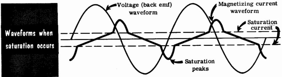
If the primary of the transformer were connected to a source of voltage having zero resistance, the sudden rise in magnetizing current due to saturation would make no difference. Drawing this heavy current from a voltage source that possesses internal resistance, however, causes a voltage drop coincident with the current peaks, distorting the primary voltage waveform as well.
