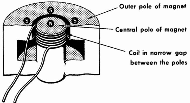
This problem is overcome, to some extent, by increasing the intensity of the magnetic field. A North and South pole are brought close together, and the wire moves in the narrow space between them. To increase its effectiveness, many turns of wire move in the same gap. It is convenient to make the gap circular, because this simplifies construction of the coil, gets the poles close together, and gives the coil free space in which to move.
