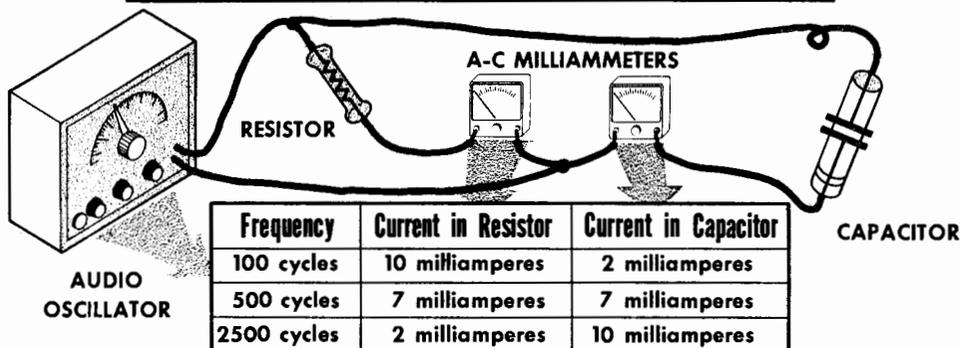
Currents of different frequencies can be separated by connecting the same components in parallel. With a resistor and capacitor in parallel, the resistor draws the current at low frequencies, the capacitor at high frequencies, and in the middle range, the current is shared. With a resistor and inductor in parallel, the resistor draws the current at high frequencies, the inductor at low frequencies, and in the middle range, the current is shared.
