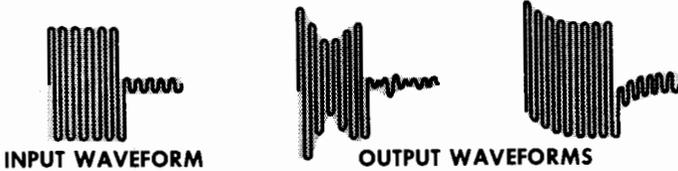
*Two Kinds of Distortion Caused by Delayed Changes Voltage*
