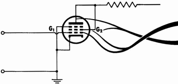
Electron flow is controlled by voltages on  $G_1$  and  $G_2$ .  $G_2$  has same voltage at all times as plate. Electrons divide between  $G_2$  and plate, but get to the same place, passing through coupling resistor.
