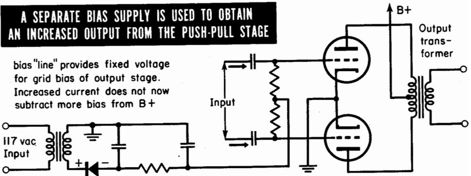
bias "line" provides fixed voltage for grid bias of output stage. Increased current does not now subtract more bias from B+
