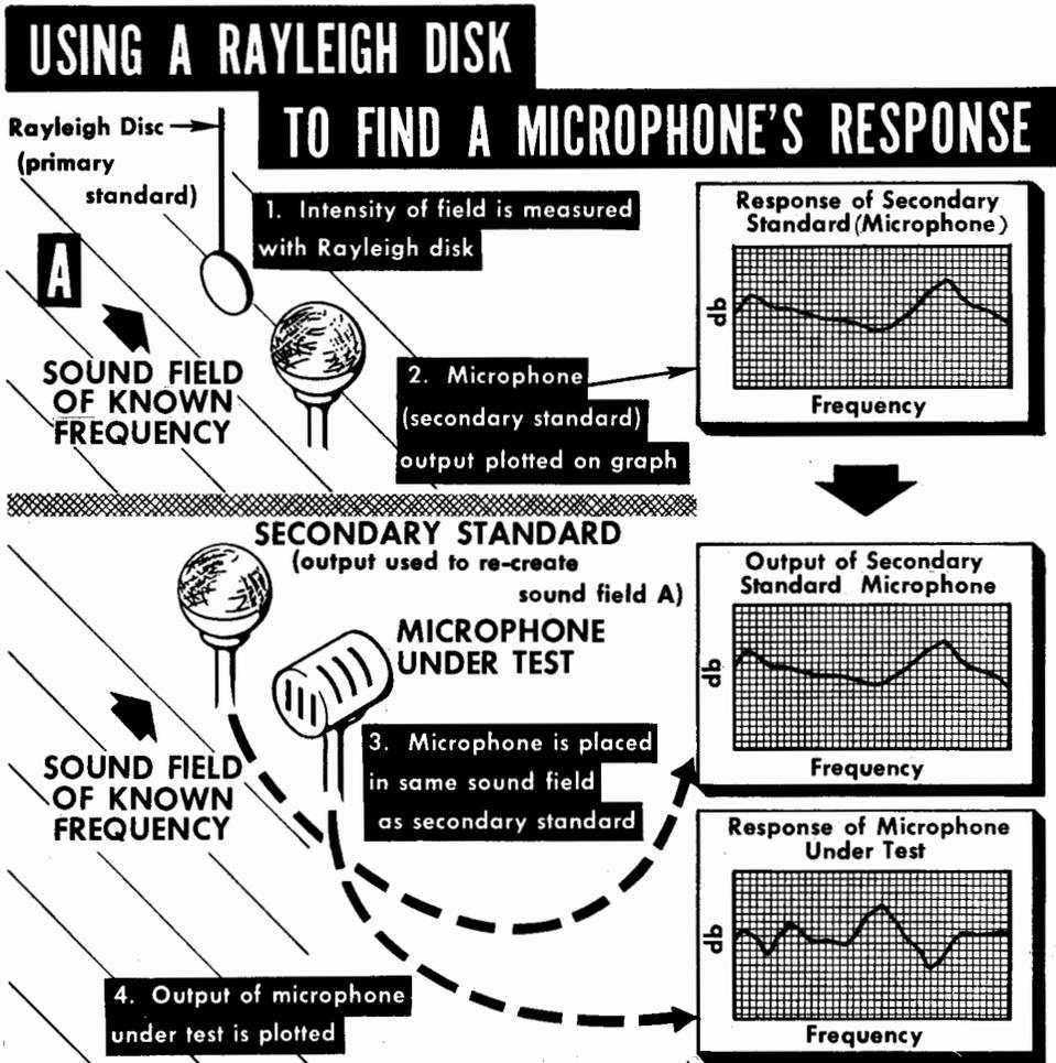
In this way we get a calibrated microphone—one with which we can measure a sound field, by making measurements and referring to its calibration chart. From this we can measure the performance of any other item of audio equipment. This calibrated microphone is called a "secondary-standard." Another microphone in the same sound field can be compared against the secondary standard, and an *absolute* response obtained for it by using the secondary standard's calibration chart.
