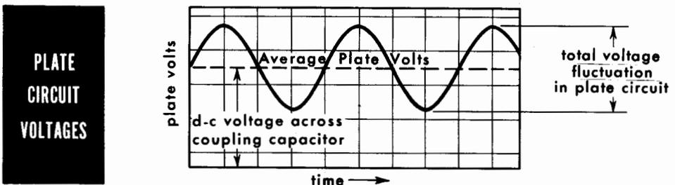
A capacitor placed between the plate and the a-c voltmeter takes on a charge corresponding to the steady or d-c component of the voltage, but does not have time to alter that charge with the alternating component. The voltmeter, therefore, measures only this alternating component.
