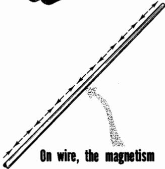
On wire, the magnetism is in alternate directions along the wire.
