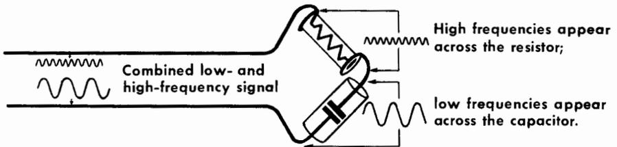
At a low frequency, the charge on the series capacitor follows the fluctuations, and the voltage across it very closely follows the input voltage, only a small current flows, and very little fluctuation appears across the resistor. At a high frequency, the charge on the capacitor does not have time to follow each fluctuation, and the whole of the applied voltage appears across the resistor.
