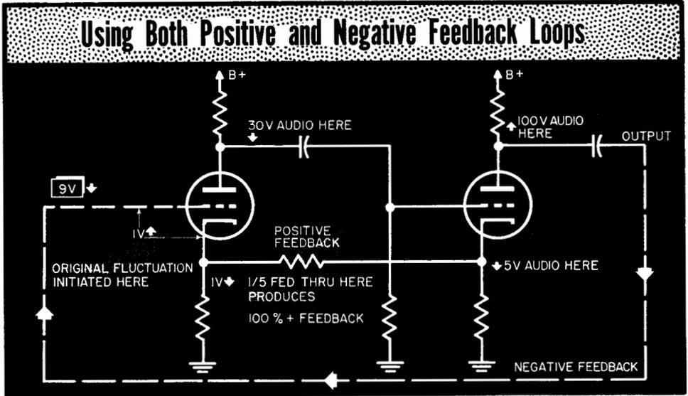
Because of amplification, positive and negative feedback, an input voltage of 9 volts is required.
