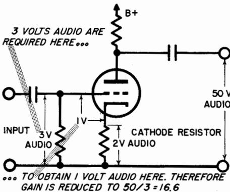
**THE CATHODE RESISTOR PROVIDES NEGATIVE FEEDBACK**
