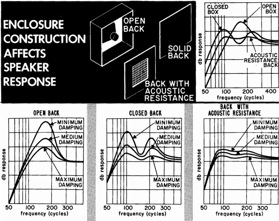
A completely open back results in a load on the diaphragm that acts as a mass or weight of air moving bodily. A completely closed back makes the air inside the cabinet act as a compressible cushion. Using an acoustic resistance consisting of a large number of holes that allow the air to pass through but offer resistance to its passage achieves an intermediate condition that damps the diaphragm properly.
