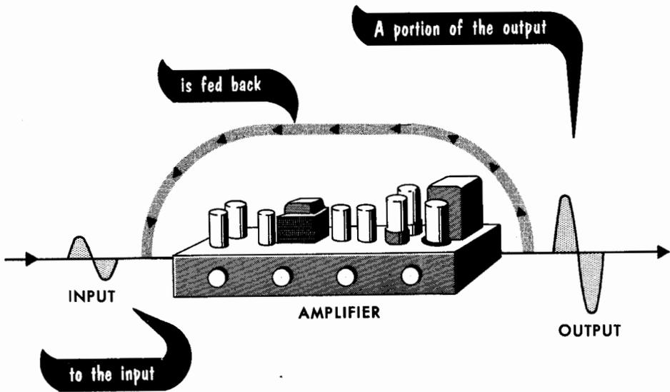
Distortion in the fed-back signal acts to reduce distortion in the output
