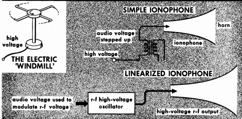
With every kind of loudspeaker, there has always been the problem of mechanical parts which can add effects of their own to the sound radiated. It has long been a dream among idealists in high-fidelity circles to find a loudspeaker which had no moving parts, but converts electrical waveforms directly into sound waves. For this reason the *ionophone* has a strong appeal.
