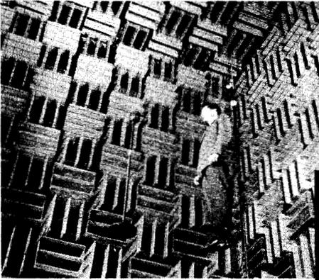
**Loss of background sounds due to excessive absorption -- such as in an Anechoic Room create a loss of perspective**
