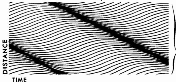
sound wave travels this far in a given time although the separate air particles only move back and forth
