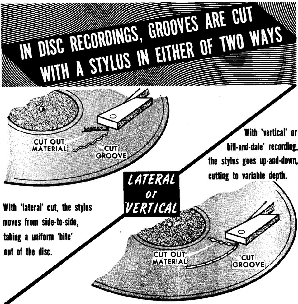
Lateral cuts are invariably used in modern recordings, because this method involves continuous removal of the same amount of material (called *swarf*) from the surface by the cutter. Vertical (hill-and-dale) cutting involves variation in the amount of material removed at the different points on the waveform, which places a varying load on the cutter. This variation in itself can cause distortion.
