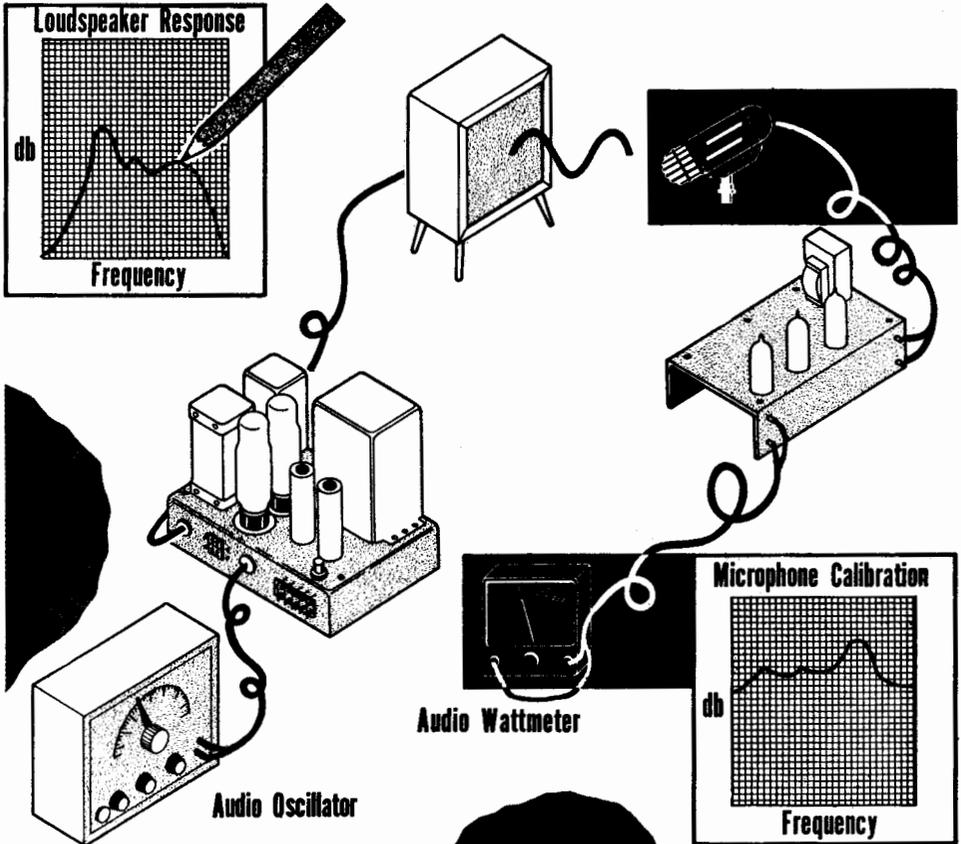
The response of a loudspeaker can also be found by using a calibrated microphone to measure the sound field that it radiates at different frequencies. For all these purposes, it is obvious that the calibrated, or secondary standard microphone should be as near perfect in response as possible, so that little correction will be necessary from its chart. High-quality condenser microphones and a special form of crystal microphone without any lever system, are favored for this purpose.
