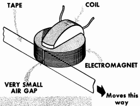
Tape and wire recording use a magnetic pattern corresponding to the audio, which is put onto a magnetic material that will hold it indefinitely. The additional track width on tape permits more magnetism to be put on it, giving a better discrimination of audio against background noise.
