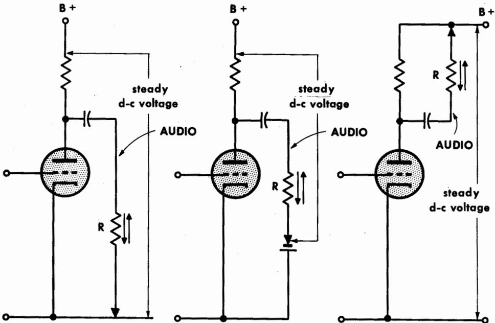
No matter where the other end of resistor R is connected, it takes the same current and voltage fluctuations from the plate
