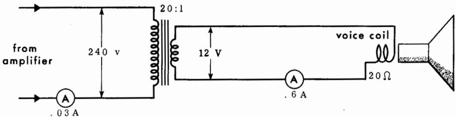
**Amplifier is NOT MATCHED to required 16-ohm, but 20-ohm speaker. Amplifier now 'sees' 8000 ohms - Output power is 7.2 Watts**
