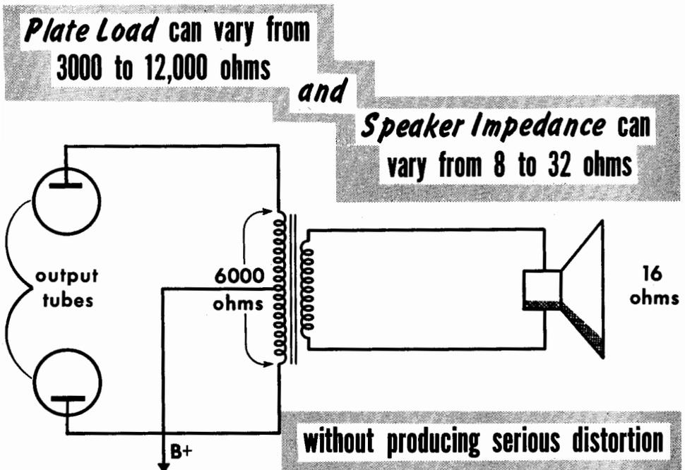
If, for example, the plate load of the two tubes in push-pull should be 6000 ohms, they will not show serious distortion if an actual plate load is used ranging from 3000 to 12,000 ohms, or even more. In terms of the secondary side of an output transformer designed to feed a 16-ohm loudspeaker, it will not produce serious distortion even if it is connected to an 8-ohm or 32-ohm loudspeaker.
