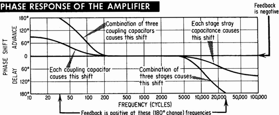
Take the effect of the coupling capacitors on the low-frequency response. If each of these capacitors produces a phase difference of  $60^\circ$  at the same frequency, the total phase shift adds up to  $180^\circ$ . This amounts to phase reversal. If the feedback starts out being negative at this particular frequency, it will convert into positive feedback.
