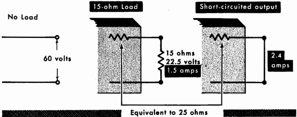
We can take the matter one stage further and consider the output with no load at all. If there is no current, there will be no feedback and a 10-millivolt input will produce  $(10/2 \times 12)$  or a 60-volt output. With the current feedback applied and a 10-millivolt input, the effective open-circuit output voltage is 60 volts, whereas the short-circuited current is 2.4 amps. This means the *effective* internal resistance is  $60/2.4$  or 25 ohms.
