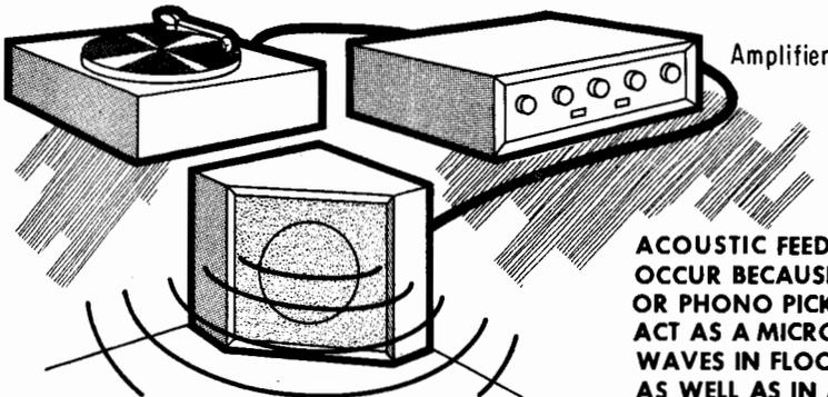
ACOUSTIC FEEDBACK MAY ALSO OCCUR BECAUSE AMPLIFIER TUBES OR PHONO PICKUPS SOMETIMES ACT AS A MICROPHONE TO SOUND WAVES IN FLOORS, WALLS, ETC., AS WELL AS IN AIR.
