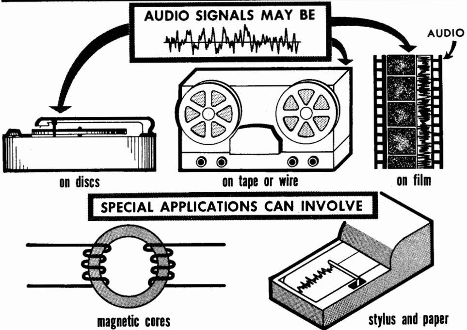
Recording plays an important part, not only in audio for high-fidelity purposes, but also in the many other applications for which modern audio equipment is used. It can be regarded as a storage medium in which long sequences of audio waveforms can be indefinitely preserved for reproducing at a later date.
