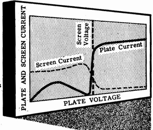
The second extra (i.e., third) grid is inserted to stop electrons from bouncing back from the plate to the screen grid when the plate potential is lower than the screen potential. If the second grid has the highest voltage of all and there were no third grid, electrons would hit the plate, cause further electrons to bounce off it, and be attracted by the more positive voltage at the screen grid. This *secondary emission* could even result in negative plate current.
