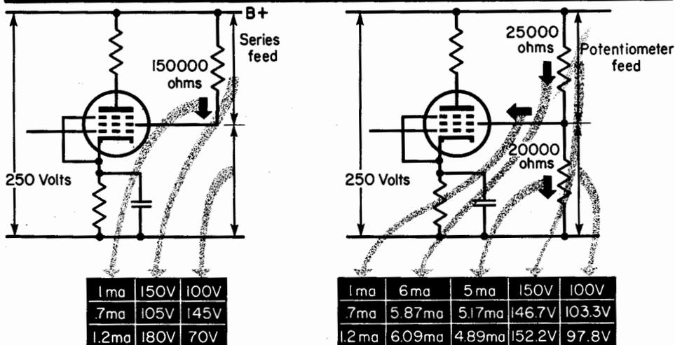
The potentiometer causes much reduced variation of screen voltage in this column for the same change of screen current in this column.
