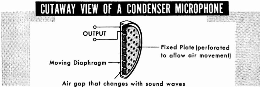
To make a condenser microphone work, it must have a steady electric charge upon it (obtained from a source of high voltage) that is isolated from the microphone so that a change in the spacing between the plates due to incident sound waves causes the voltage between them to go up and down. This is done by connecting a high voltage across the plates through a large resistance. The fluctuating voltage due to sound waves is fed through a coupling capacitor to an output resistor.
